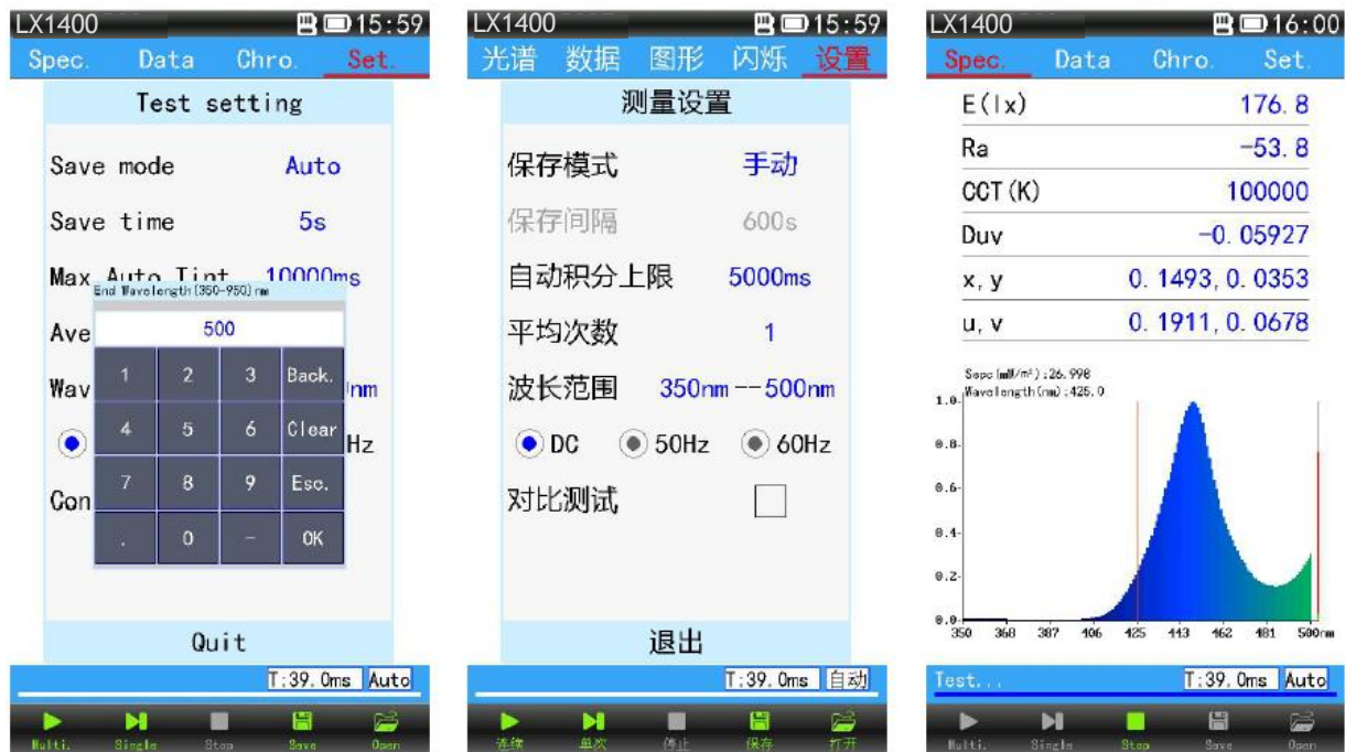
Wavelength measurement range setting
